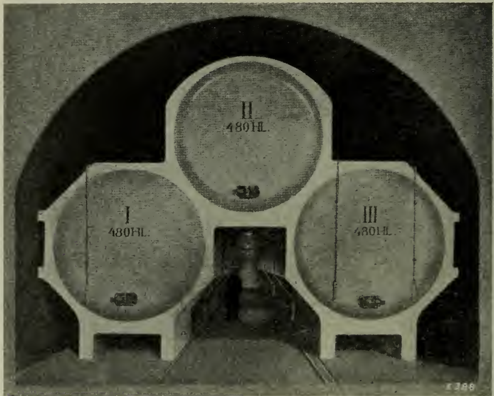
FIG. 4. CYLINDRICAL VATS. TOTAL CAPACITY, 100,000 GALLONS.
